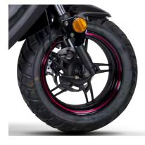
The correct tire pressure is essential for the safety and driving of the scooter. Tire pressure should be checked before each use. While driving the scooter, tire temperature and pressure will change depending on speed and load. For this reason, tire pressure should only be checked and adjusted when the tires are cold. Normal tire pressure (cold)
