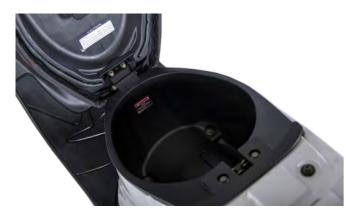
Use the key switch lock to unlock the saddle to open the luggage compartment. The lock is located on the left rear fairing. To lock the saddle, lower it until it clicks. Make sure the saddle is securely locked before riding the scooter. In the luggage compartment you will also find a tool kit
